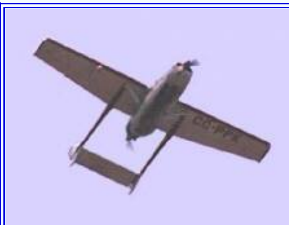
The Cessna 337 Skymaster (also shown below, with optional belly pod) tried to solve the light twin's typical
